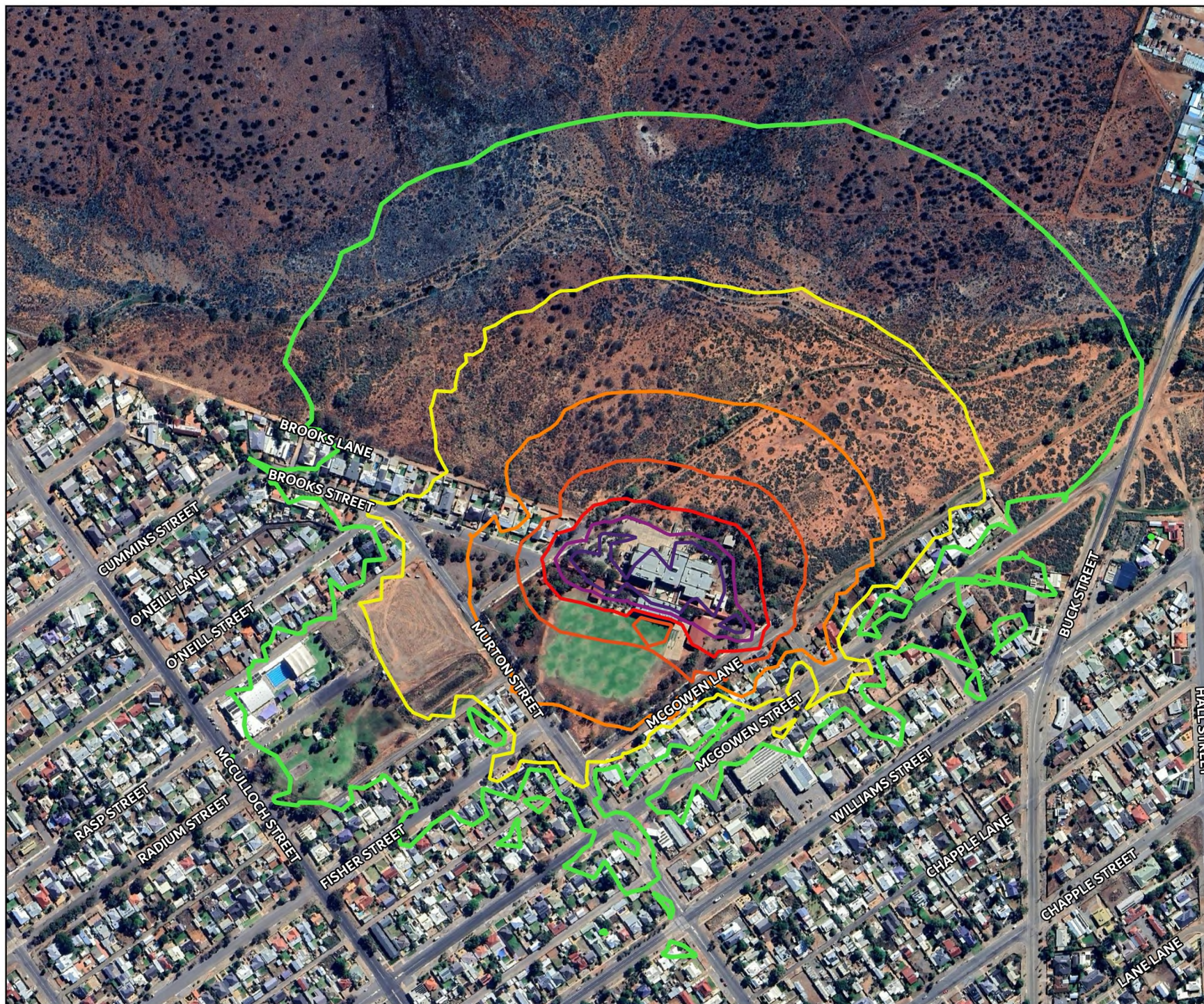
FIGURE 6 Noise contours Scenario 3 - Structural Demolition MAC252351-01 WILLYAMA HS DEMOLITION
