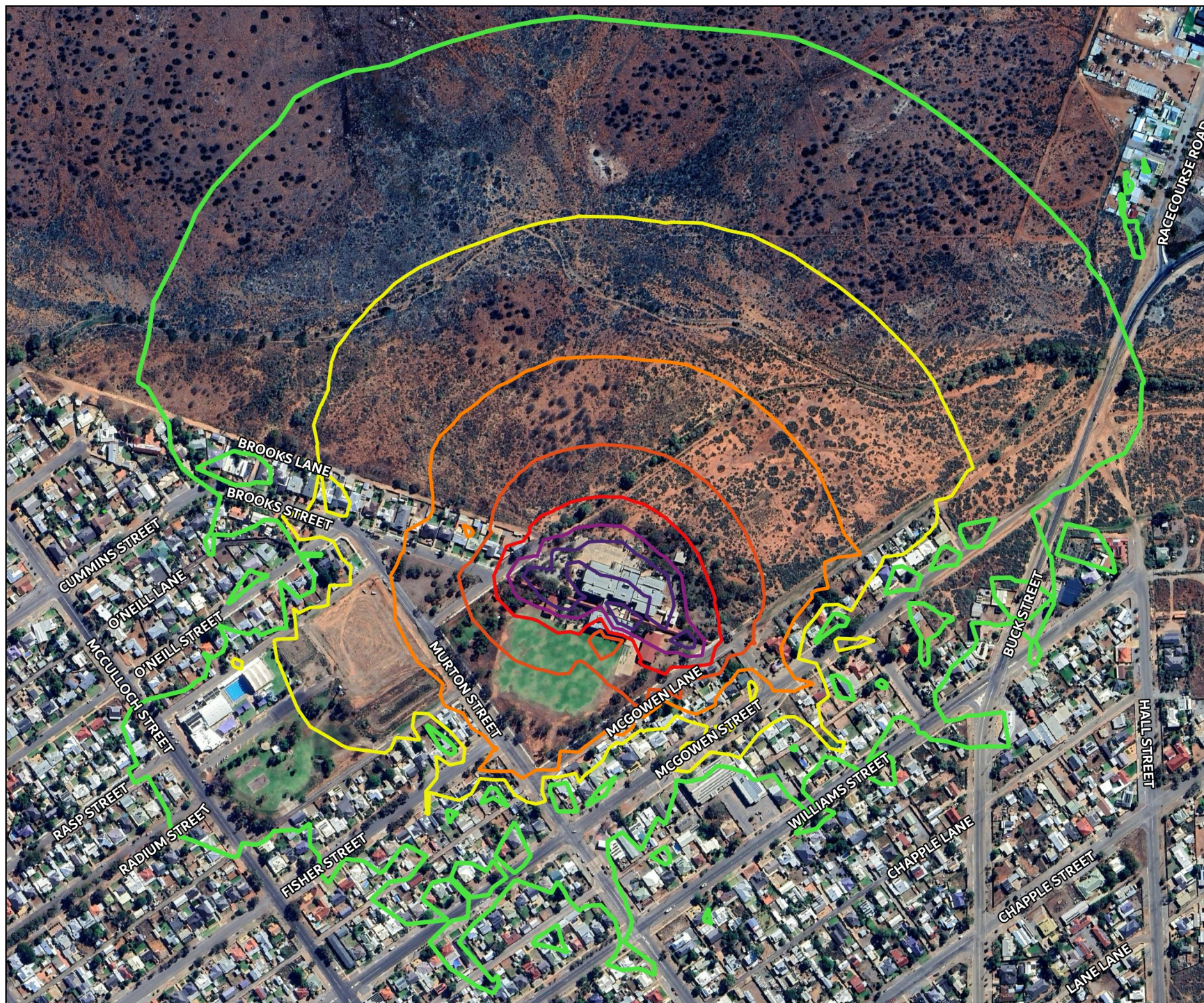
FIGURE 7 Noise contours Scenario 3 - Structural Demolition with Crushing MAC252351-01 WILLYAMA HS DEMOLITION
